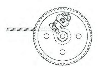
When inserting the lifting cable into the drum, insert it into the correct end of the hole as shown above. Tighten the set screw securely.
