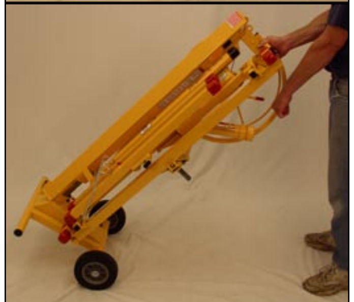
Handle the loaded PANELLIFT® Model 110 Drywall Lift Cart as you would any two wheel material handling dolly.
