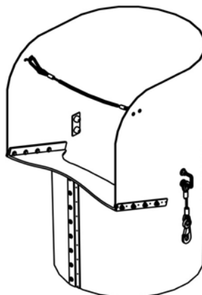
Polyethylene Kickboard Thickness: 3/8" (9 mm)
