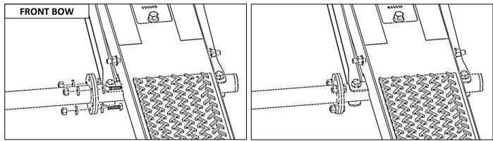
• Using three more 1/4" x 7/8" hex head screws, 1/4" washers, and 1/4" lock nuts, attach the opposite end of the torsion tube extension to the torsion tube as shown below.
