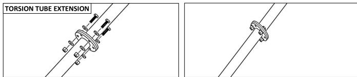
• Using three more 1/4" x 7/8" hex head screws, 1/4" washers, and 1/4" lock nuts, attach the opposite end of the torsion tube to the rear bow as shown below.
