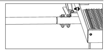
• Attach handle into operator arm by pushing handle in and then pulling out.
