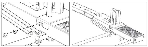
If using an extension ladder put the ladder stop at the same location on the front & rear bow assembly.
