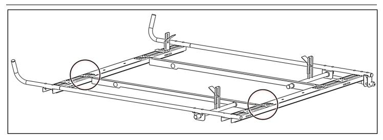
Attach the long L-bracket to both bows in the orientation shown using 3/8" x 1" carriage bolts, 3/8" flat washers and 3/8" lock nuts.
