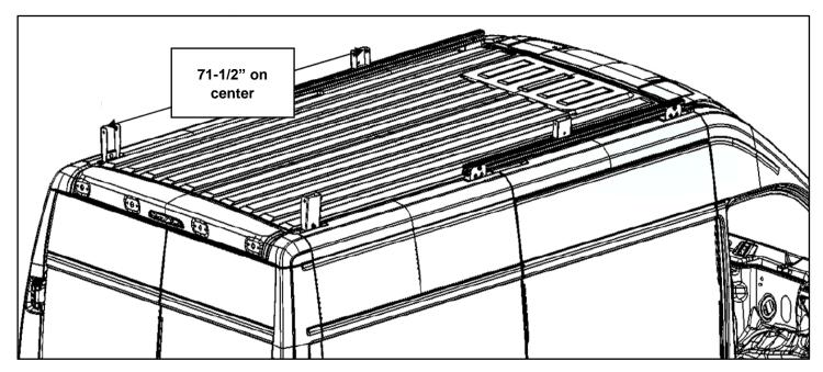
If using the optional ladder rack extender, set the center-to-center distance between rear and front feet to 96".
