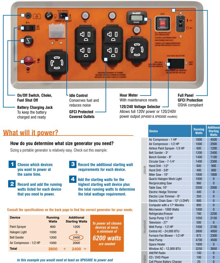
In this example you would need at least an XP6500E to power and start all of these devices at one time because an XP6500 provides 6500 running watts and 8125 starting watts.
