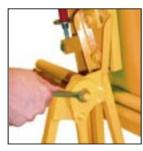
When properly adjusted the Tilt Handle will move and hold a door at any point within the full range of travel. To hold securely, the Tilt Handle must be adjusted to produce sufficient drag between the friction surfaces of the discs within the Tilt Handle mechanism. To increase or decrease drag on the Tilt Handle: Tighten or loosen the two lock nuts as needed. Note: Friction disc surfaces are to remain clean and dry. Do not lubricate with oil.
