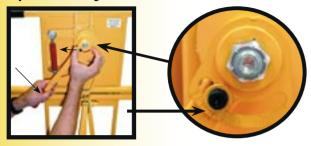
Important! The Lift Handle must move freely in both directions when controlled by the operator. If handle drifts by itself and fails to hold the door at the desired elevation or if the handle won't rotate clockwise to lower the door -STOP!
