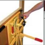
Max. Load: 160 lbs. (72 kg) Max. Door Height 7' (213 cm) Max. Door Width 4' (121.9 cm)
