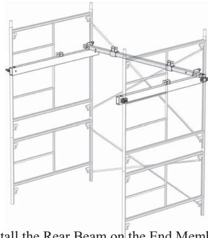
Install the Rear Beam on the End Members.
