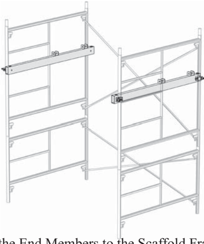
Attach the End Members to the Scaffold Frames.
