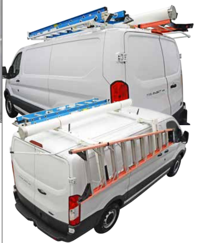
COMBO RACKS WITH BOTH EZ LO-DOWN AND CLAMP & LOCK UNITS ARE AVAILABLE FOR LOW ROOF AND COMPACT VANS.
