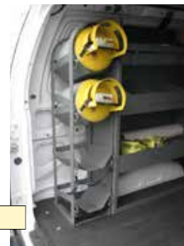
40100 4 Tier Refrigerant Tank Rack
